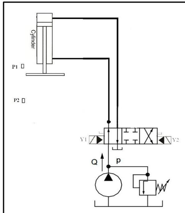
Figure 1. hydraulic system diagram
