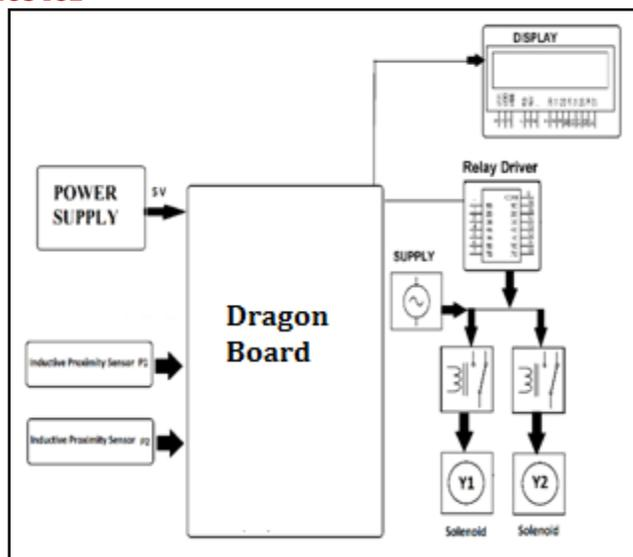
*Figure 2 Basic Connection of Dragon Board with Sensors and Relays*
